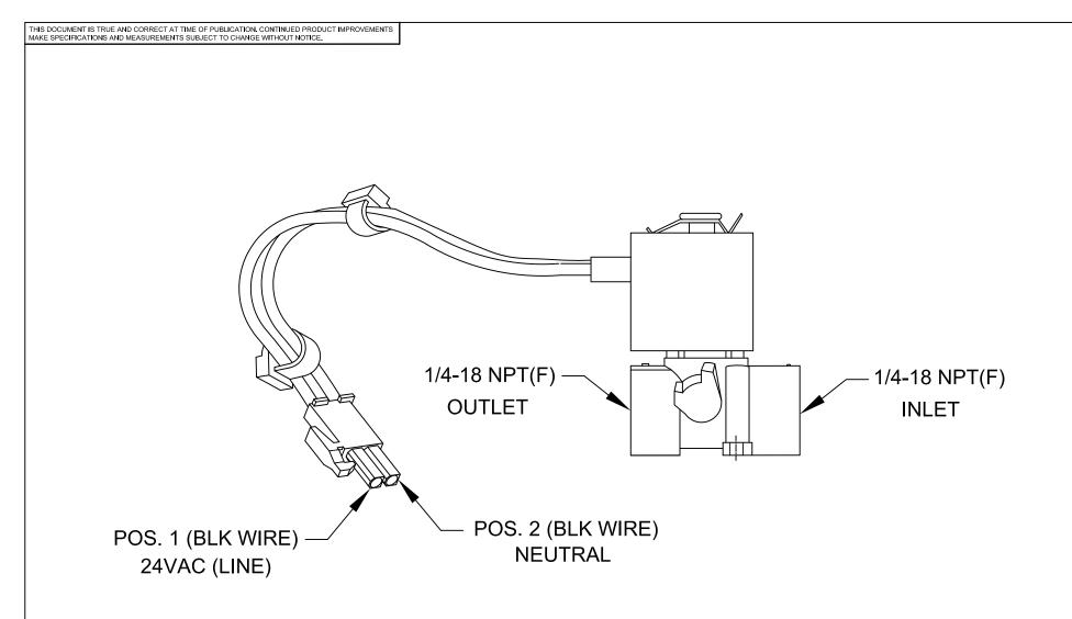
\* MUST BE USED IN CONJUNCTION WITH 24VAC TRANSFORMER AND SENSOR
