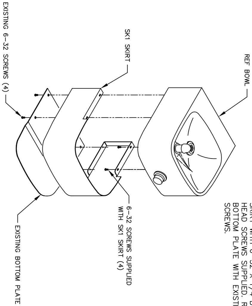
\*\* REMOVE BOTTOM PLATE. ATTACH SKIRT WITH 6-32 X 1/4 BUTTON HEAD SCREWS SUPPLIED. REATTACH BOTTOM PLATE WITH EXISTING 6-32 SCREWS.
