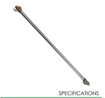
Model MK81A is a special freeze-protected valve that drains water from Model 8300FP combination shower/eyewash after closing to prevent freezing. 1-1/4" MIPS inlet. Standard sizes are 60" and 78" (152.4 and 198.1 cm) for bury depths of 24" and 42" (61 and 106.7 cm) respectively. Servicing Instructions: For replacement of damaged parts, order the VRKMK81A repair kit which includes packing, stuffing box, stuffing box nut, spring and plunger assembly with four O-rings.
