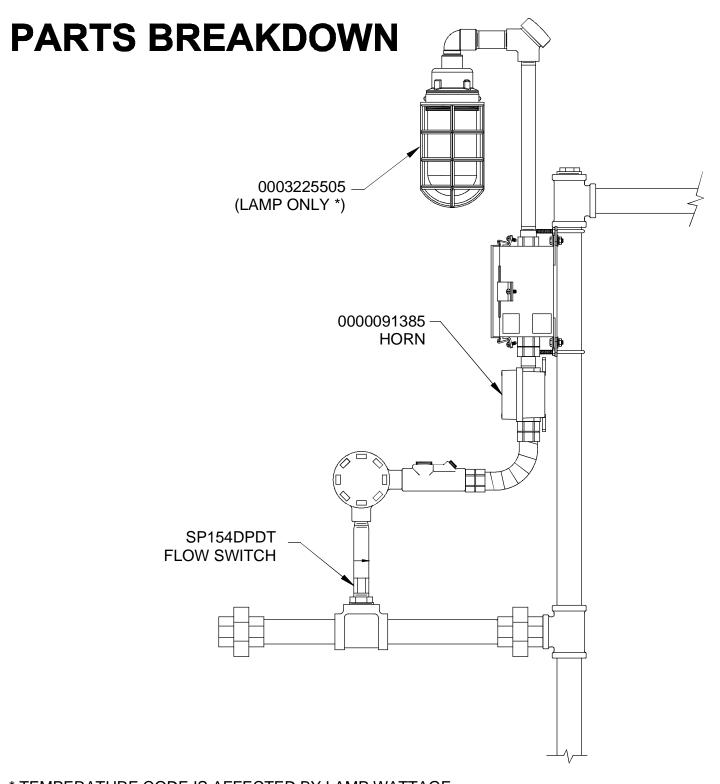
\* TEMPERATURE CODE IS AFFECTED BY LAMP WATTAGE. RECOMMENDED 60 WATT LAMP YIELDS T2C (230 DEG C), 150 WATT YIELDS T2 (300 DEG C).
