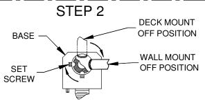
NOTE DEPTH OF SET SCREW PRIOR TO LOOSENING.
