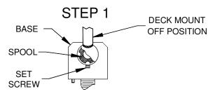
UNIT IS SHIPPED IN DECK MOUNT CONFIGURATION. TO CONVERT TO WALL MOUNT CONFIGURATION, POSITION ARM IN "DECK MOUNT OFF POSITION" AS ABOVE.
