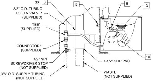
\*NOTE: TEE SHOWN ASSEMBLED FOR REFERENCE ONLY. POSITION TEE AND TRIM TUBING AS NEEDED TO FIT INSTALLATION APPLICATION.
