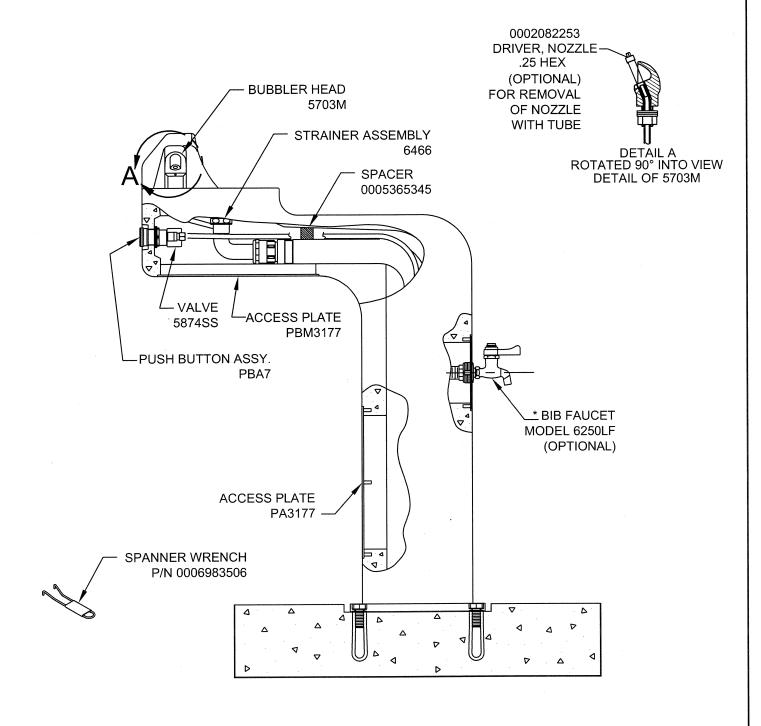
\* NOTE: MODEL 6250LF MUST BE USED WITH ACCESS PLATE 0004499489
